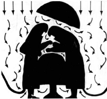
Fig. 7. Semitransparent air flow combined with body exhaust system. Turbulence not sufficient to permit currents rising from the floor. Perfect overhead surgical lighting possible.
